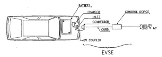
Electric Vehicle Supply Equipment (EVSE) consists of the connector, cord, and interface to utility power. Currently the interface between the EVSE and utility power will be directly hard-wired to the control device, and each automake has its own EVSE design.
