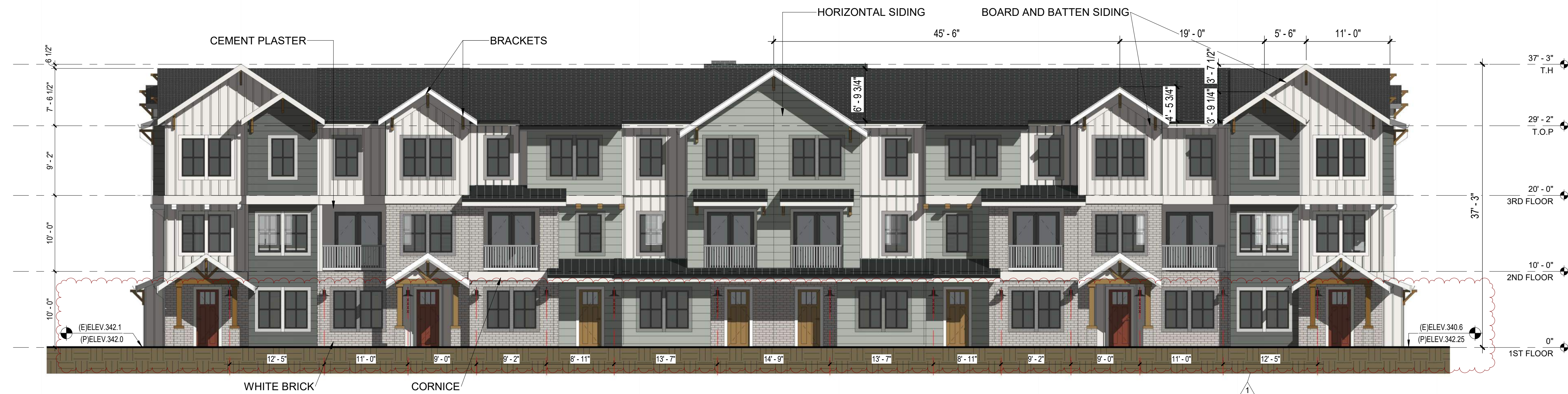
A BUILDING 1 - SOUTH ELEVATION 1/8" = 1'-0"
