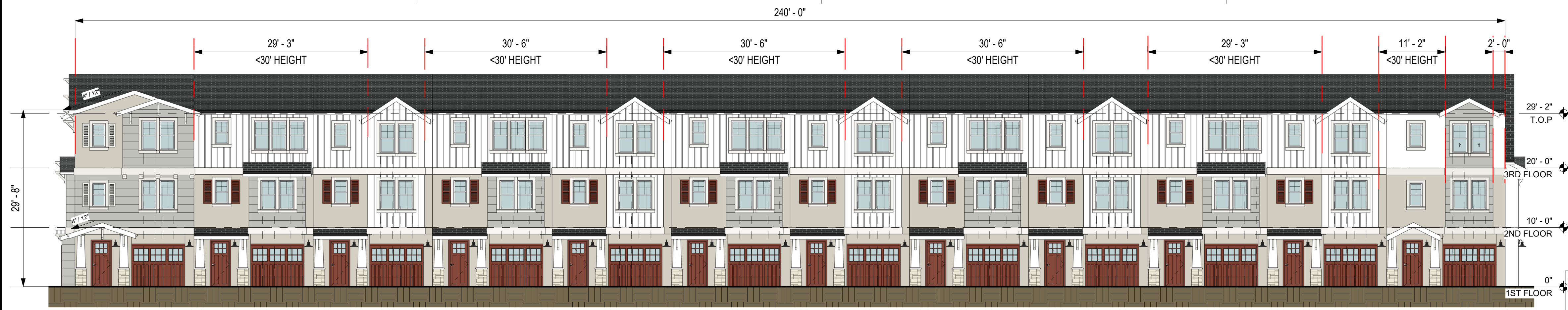
1 BUILDING 5 - WEST ELEVATION - AERIAL ACCESS CALCULATION 3/32" = 1'-0"
