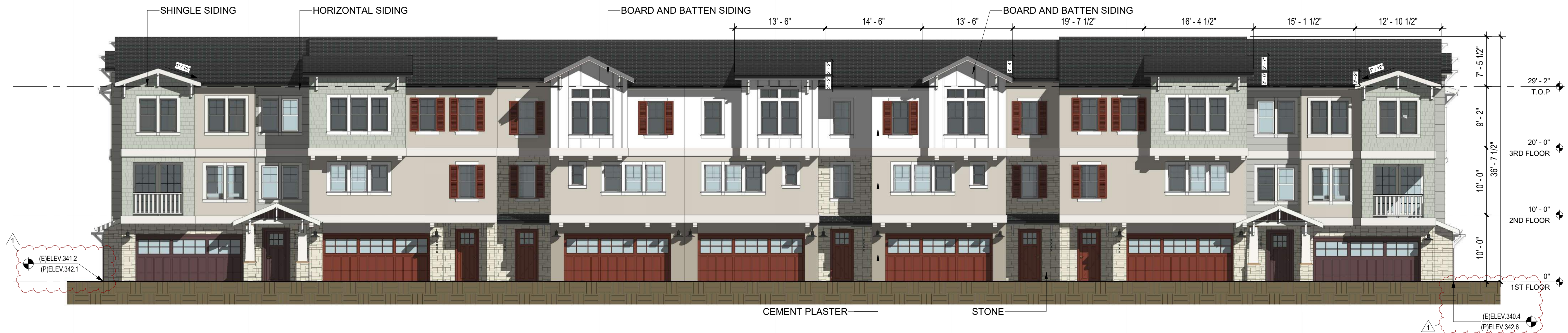
B BUILDING 6 - EAST ELEVATION 1/8" = 1'-0"
