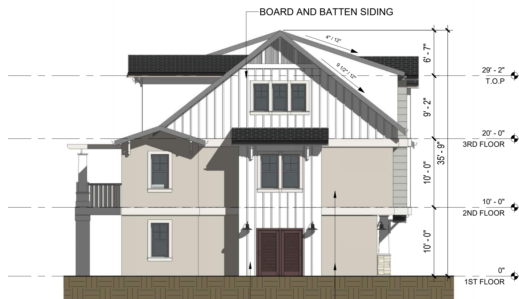
C BUILDING 8 - EAST ELEVATION 1/8" = 1'-0"
