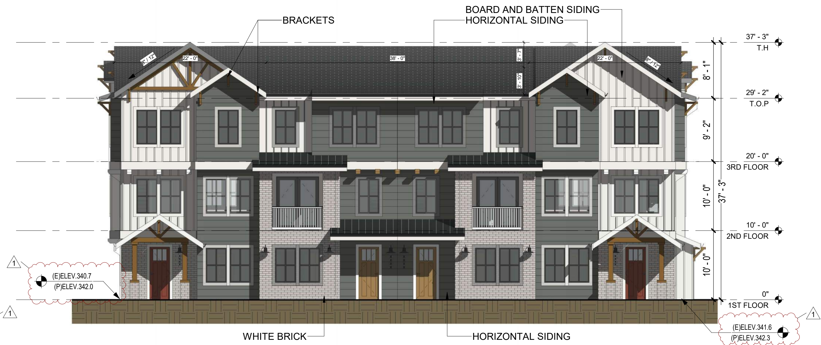
B BUILDING 9 - WEST ELEVATION 1/8" = 1'-0"
