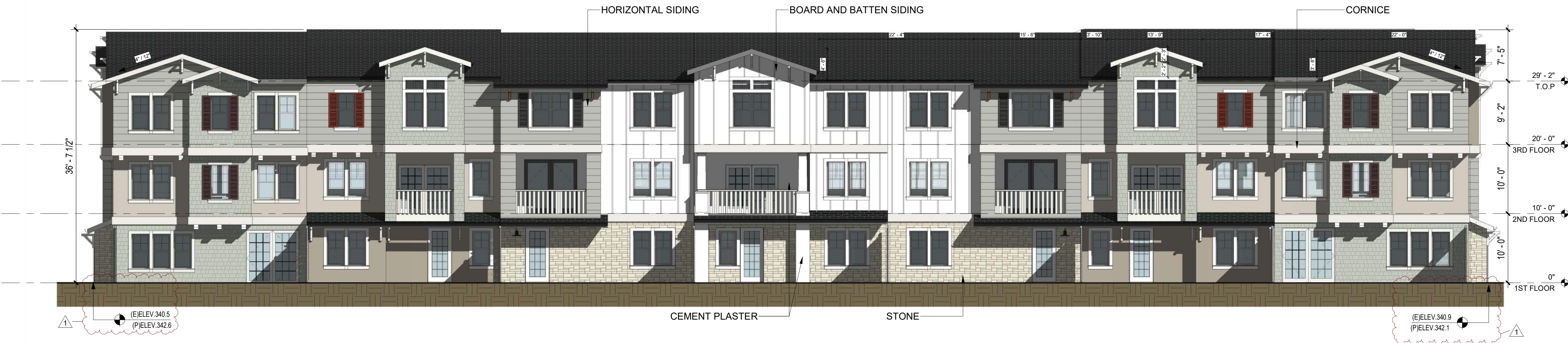
A BUILDING 6 - WEST ELEVATION 1/8" = 1'-0"
