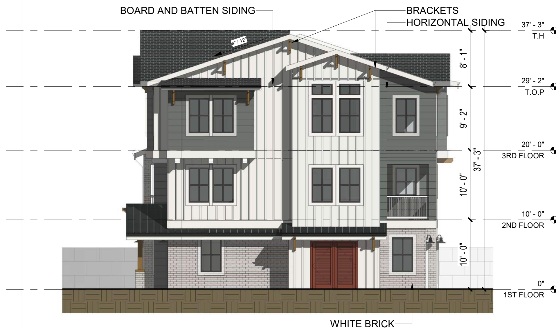
C BUILDING 9 - SOUTH ELEVATION 1/8" = 1'-0"
