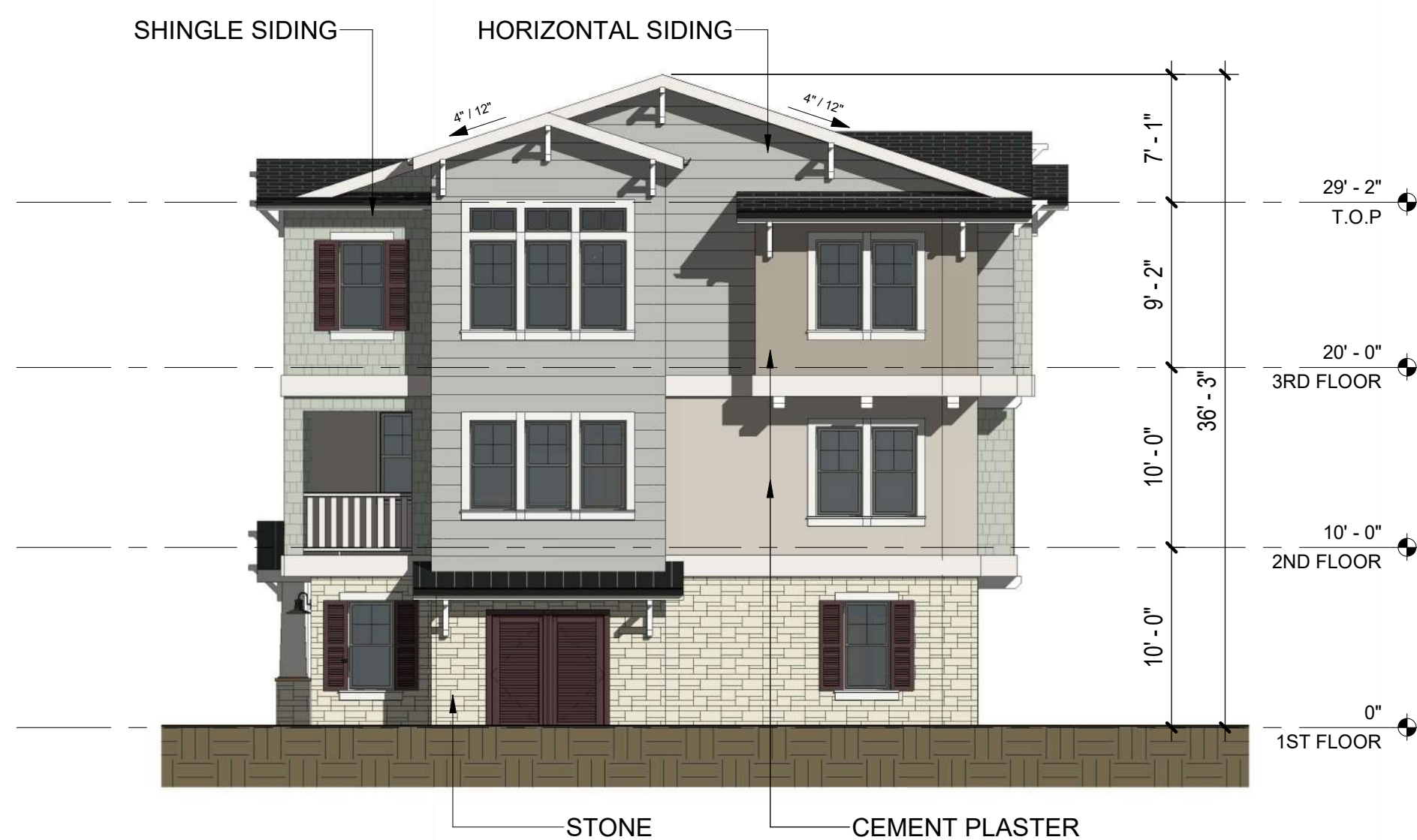
C BUILDING 6 - NORTH ELEVATION 1/8" = 1'-0"
