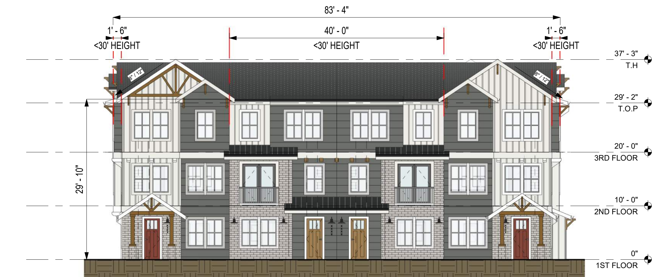
6 BUILDING 9 - WEST ELEVATION - AERIAL ACCESS CALCULATION 3/32" = 1'-0"
