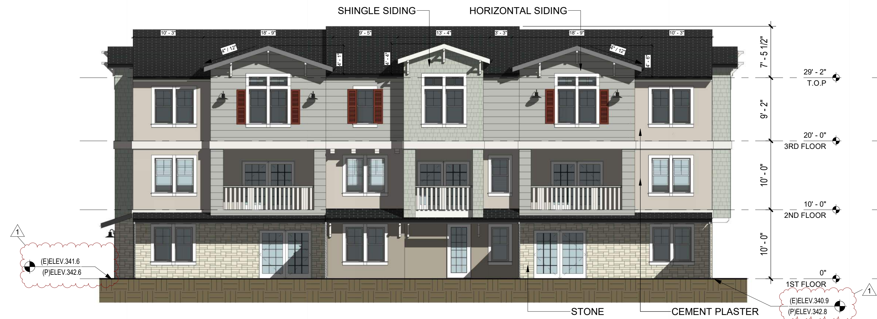
A BUILDING 7 - NORTH ELEVATION 1/8" = 1'-0"
