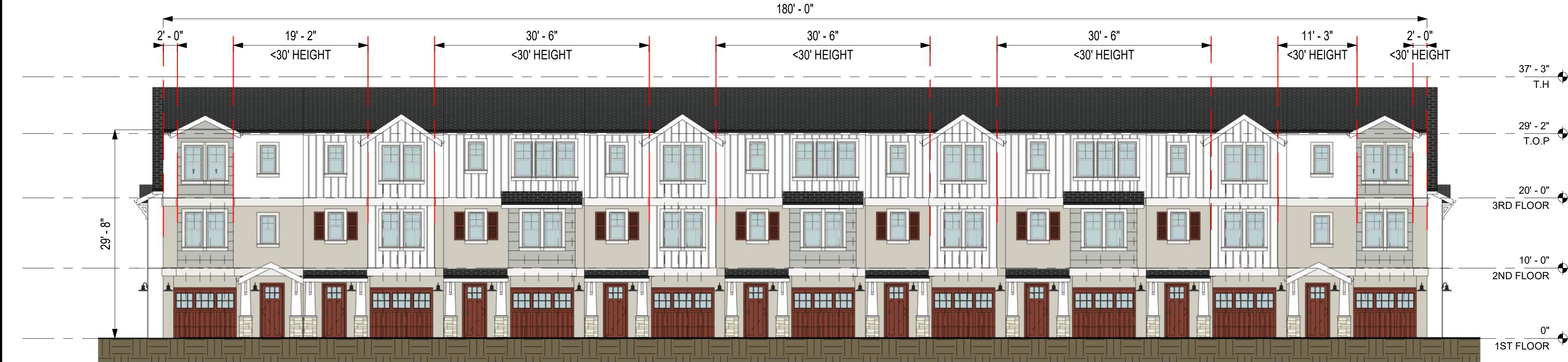
3 BUILDING 8 - NORTH ELEVATION - AERIAL ACCESS CALCULATION 3/32" = 1'-0"
