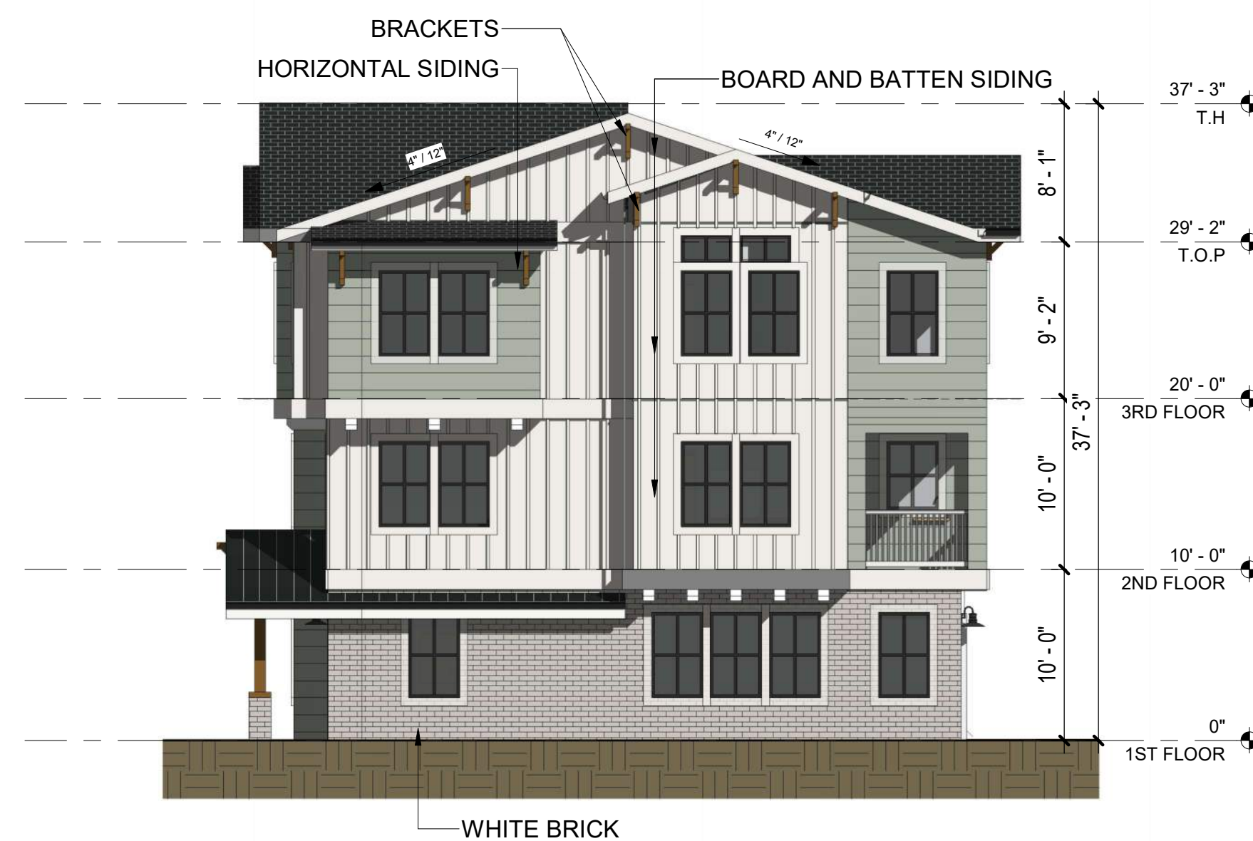
D BUILDING 10 - NORTH ELEVATION 1/8" = 1'-0"
