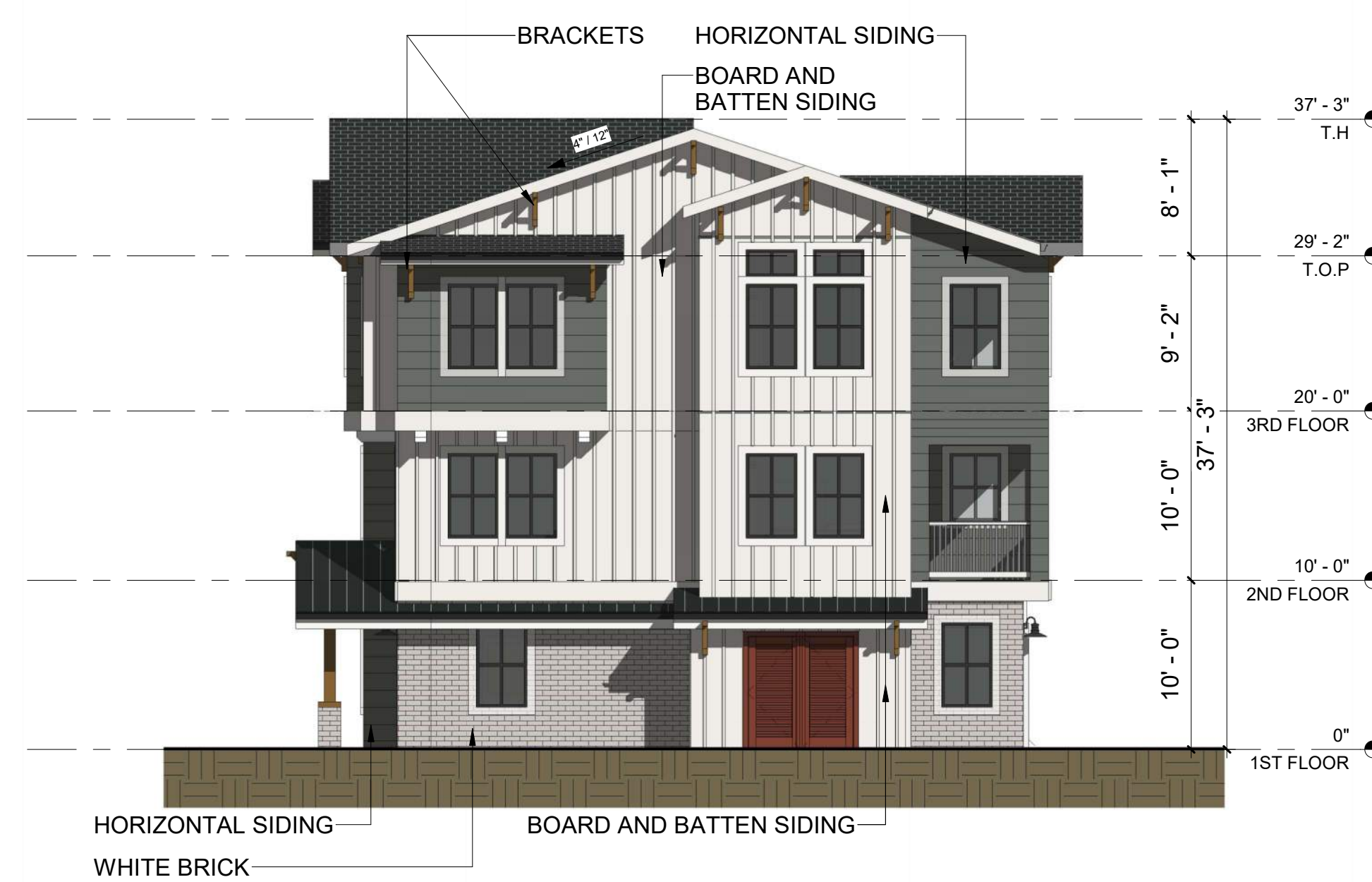
(D) BUILDING 4 - SOUTH ELEVATIONS 1/8" = 1'-0"
