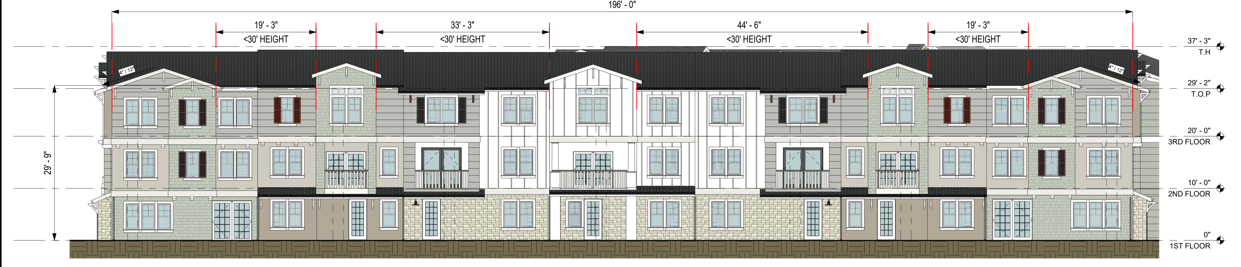
4 BUILDING 6 - WEST ELEVATION - AERIAL ACCESS CALCULATION 3/32" = 1'-0"
