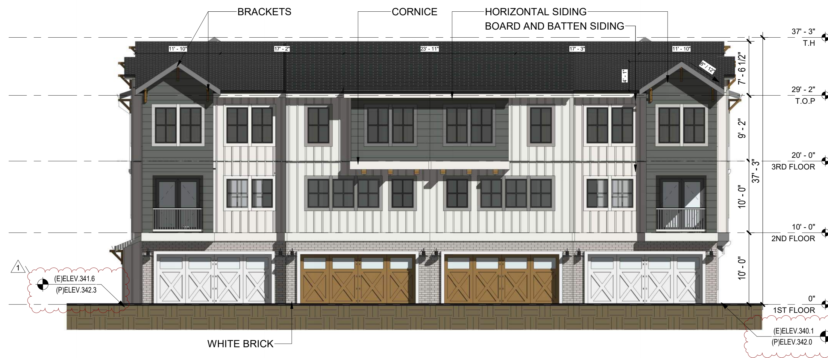
A BUILDING 9 - EAST ELEVATION 1/8" = 1'-0"
