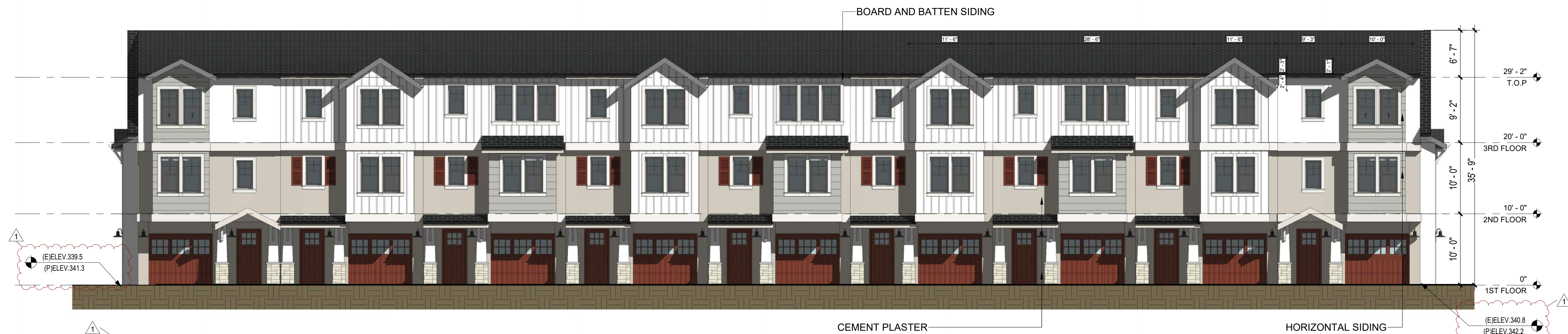
B BUILDING 8 - NORTH ELEVATION 1/8" = 1'-0"
