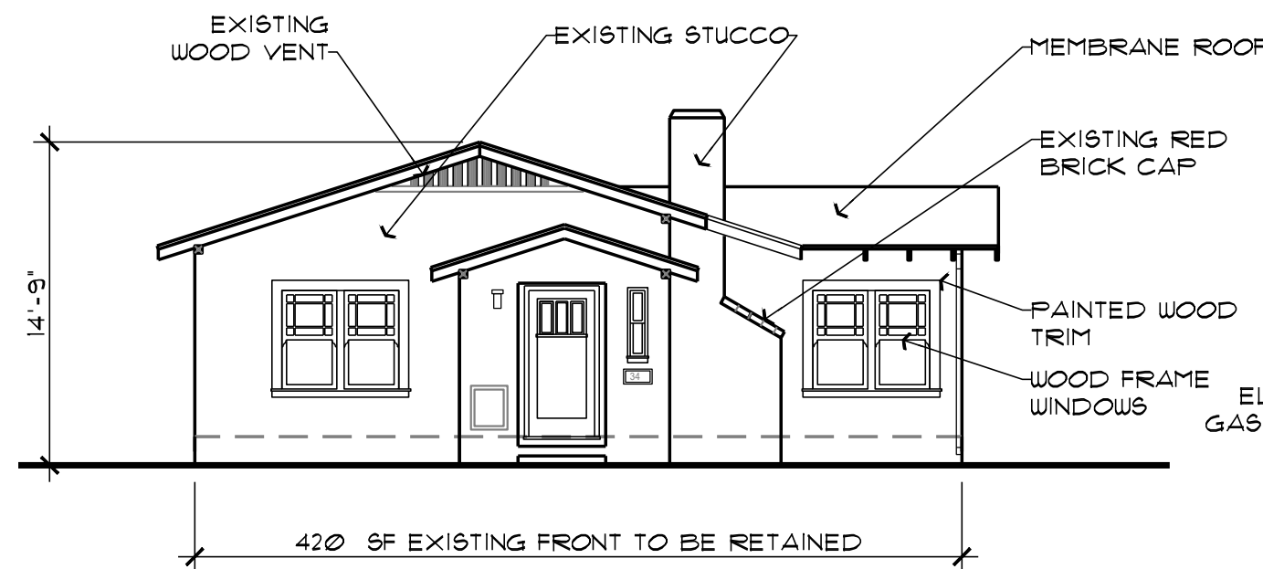
EXISTING WEST ELEVATION
