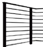
4 custom railing: dark grey 2"x3" tube steel frame with 5/8" metal rod infill height 36" posts: 3"x2" dark grey tube steel height 8'-0"
