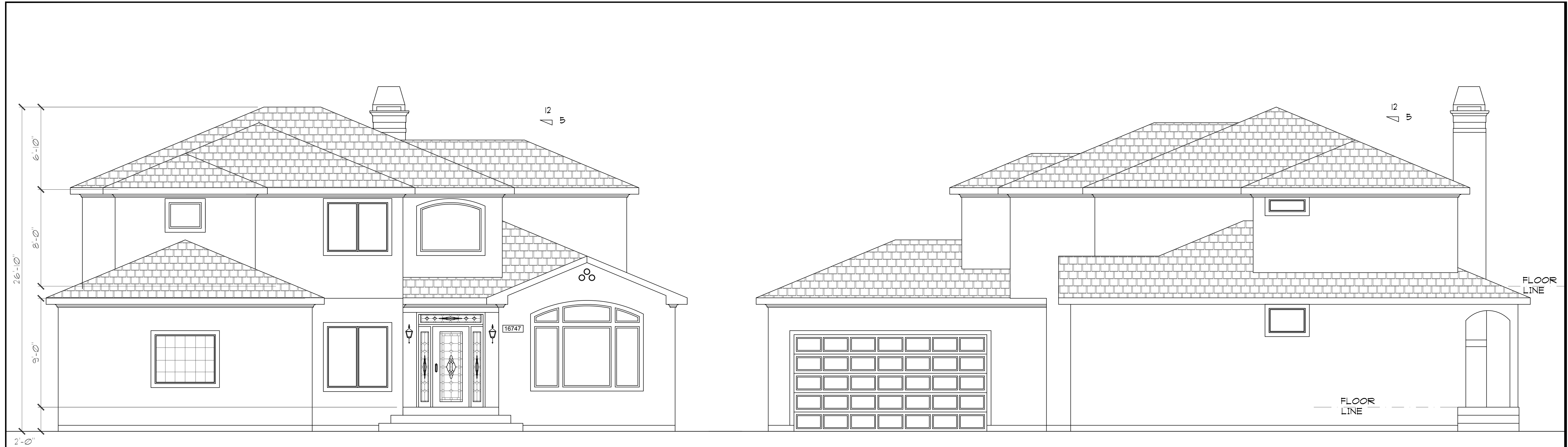
PROPOSED FRONT ELEVATION 1/4" = 1'-0"
