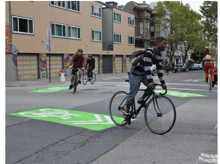
Example of green-backed sharrows
